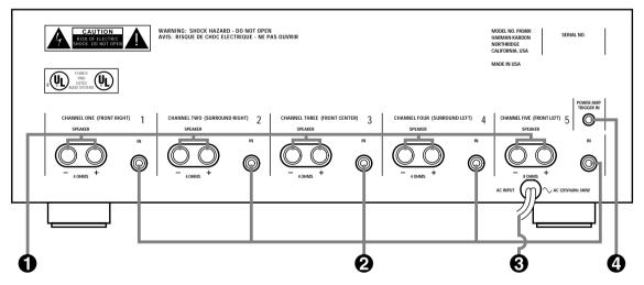
**()** Speaker Outputs: Connections from these terminals should be made to the appropriate speakers in your system.
